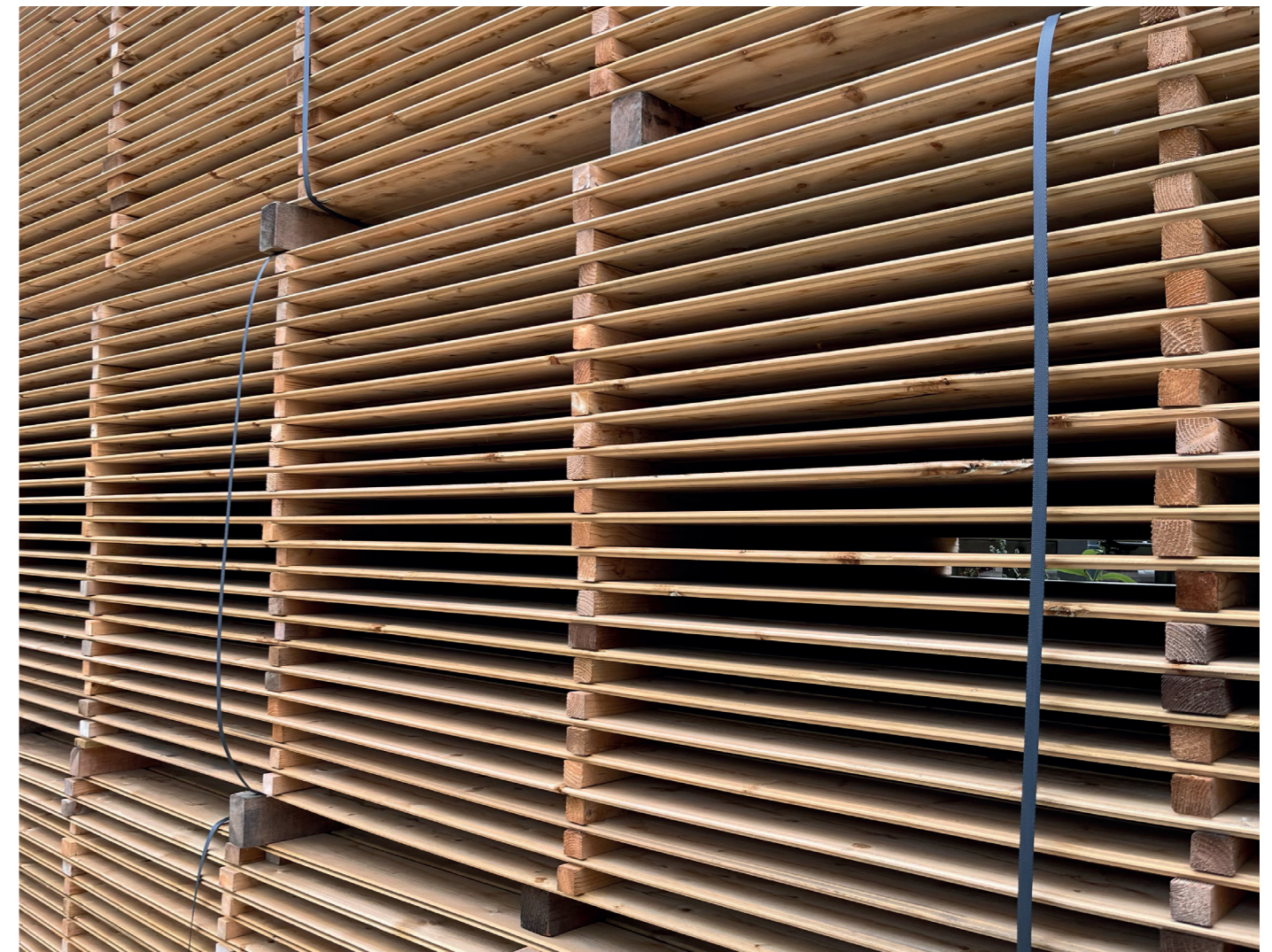
Latted timber drying process
